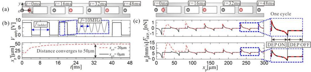
Figure 2: (a) The schematic of time series variation of particles' positions, (b) the relative positions of the particles initially located at  $x_{p,0}=0$  and  $20\mu\text{m}$  at  $t=0\text{s}$  and the applied low frequency oscillation, and (c) the  $F_{DEP}$  applied to the particles in these two cases and their streamwise velocities.
