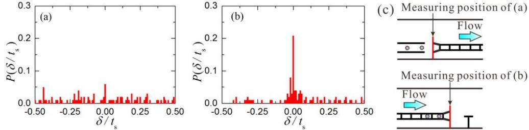
Figure 4: Probability density distributions of the deviation of the particles  $\delta$  from the synchronized time at the (a) inlet and (b) outlet, and (c) schematics of the measuring positions.
