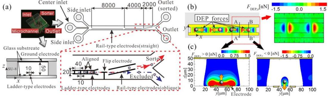
Figure 1: Schematics of (a) the microchannel, (b)  $F_{DEP,x}$  on the  $x$ - $y$  plane at  $z=6\mu\text{m}$  and (c)  $F_{DEP,z}>0$  on the  $y$ - $z$  plane (A-A' plane of (b)) and  $F_{DEP,z}<0$  on the  $y$ - $z$  plane (B-B' plane of (b)).
