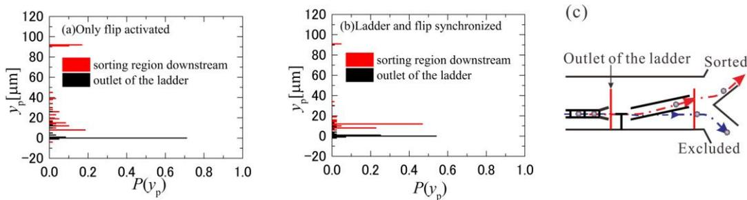
Figure 5: Probability density distributions of the particles spanwise positions  $y_p$  at the outlets of the ladder-type electrodes and the sorting region in the cases of (a) non-activated (only flip activated) and (b) activated (ladder and flip synchronized). (c) shows the measuring points of these two locations.
